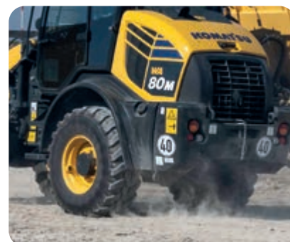
40 km/h limited hydrostatic driveline (option)
