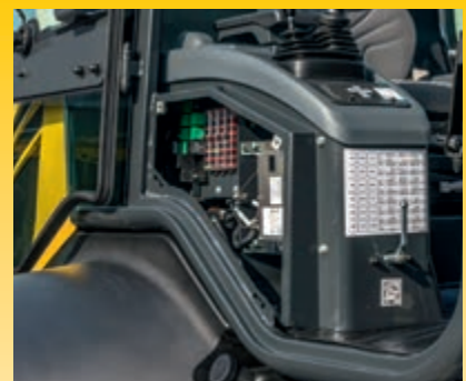
Side cover for quick maintenance access
