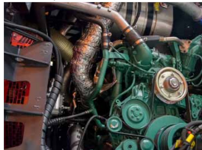
Moteur Volvo Penta (E U Stage IV/V, 13L, 390 kW, 530 HP @ 1900 Tours/min.)
