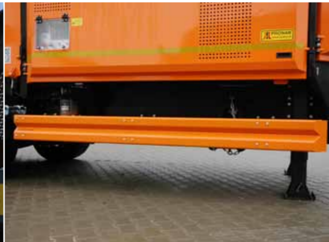
Protections anti-encastrant en acier
